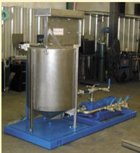
This new suspension batch mixing plant, funded by SAGIT, will be used to produce experimental suspension fertilisers for testing on EP and other areas of SA.
